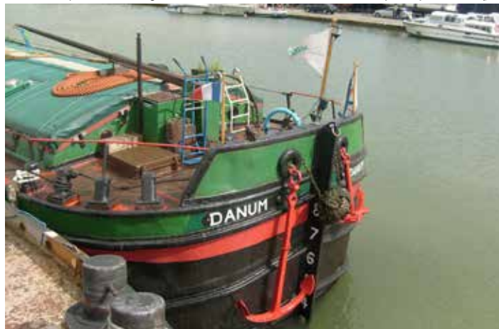
The bluff bows of a Humber keel: the orange tow-rope, the fisherman's anchor, the hessian bow-fender were part of her gear in the 1930s
